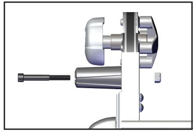
2. Using a 1/2" wrench and a 1/4" Allen wrench, remove and discard the existing nut, bolt, and bumper. Then, replace with new parts and tighten firmly into place.
